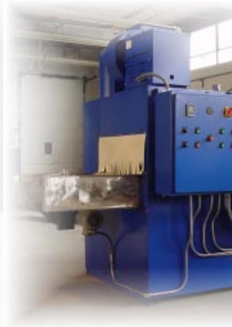
*Gas fired two-stage wash & dry system.*
