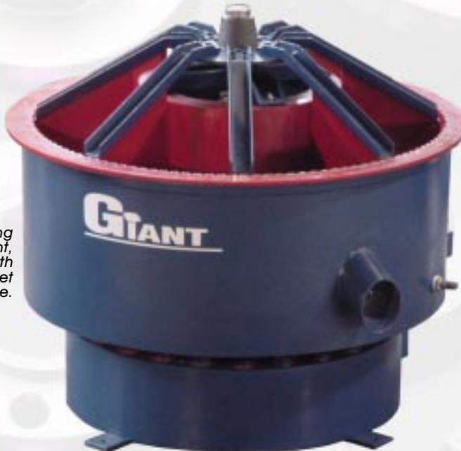
Giant Finishing makes four cost-effective bowl units - flat or spiral bottom belt drive and flat or spiral bottom direct drive - for an unlimited range of batch applications.
